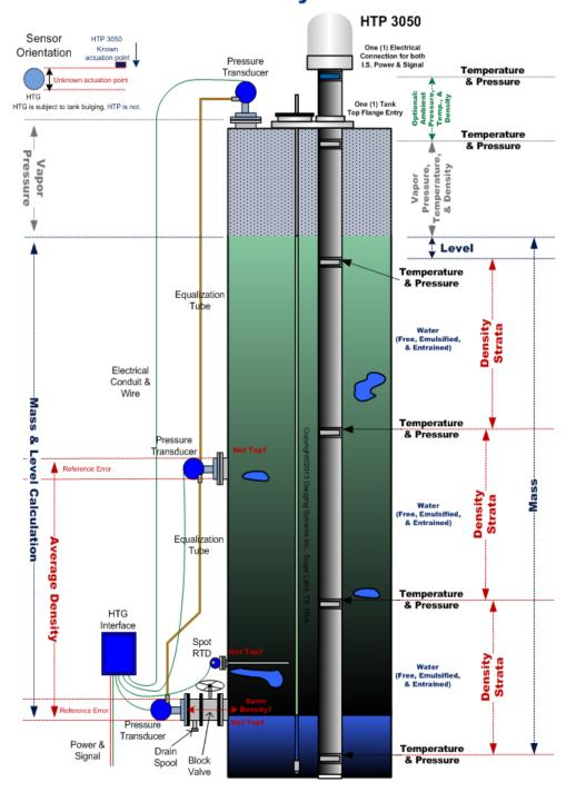
Volume by Hydrostatic Method - API MPMS Chapter 16.2
